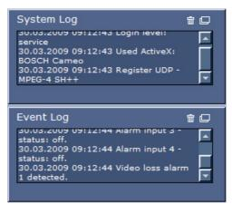
The **System Log** field contains information about the operating status of the VideoJet X10 SN and the connection. You can save these messages automatically in a file (see *Section 5.15 Advanced Mode: LIVEPAGE Functions, page 42*).
